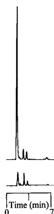
Figure 2. Chromatograms (top and bottom) showing the adsorption of 2-naphthoxyacetic acid before and after the process on the fraction of humic acids obtained under acidic conditions. The percentage of adsorption was estimated to be 94% for a time period of 3 h. Refer to Table 1 for chromatographic conditions and data.
