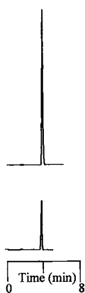
Figure 3. Chromatograms (top and bottom) showing the adsorption of phenoxyacetic acid before and after the process on the fraction of humic acids obtained under basic conditions. The percentage of adsorption was estimated to be only 51% over 3 h. However, the percent adsorption was as high as 81% on the fraction of humic acids collected under acidic conditions over the same time period (refer to Table 1 for data).
